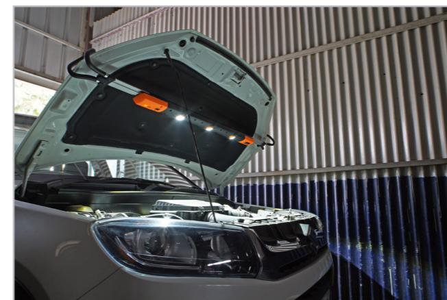
Light bulbs pivot independently to direct light as needed
